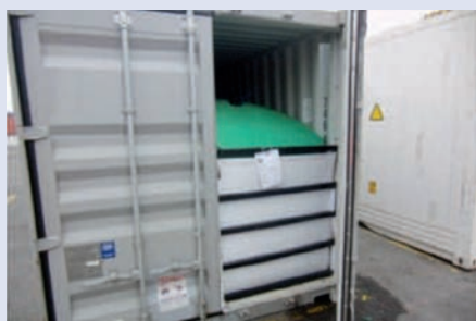
Container fitted with flexitank
