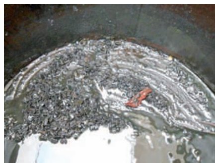
Waxy sediment/sludge at the bottom of the tank
