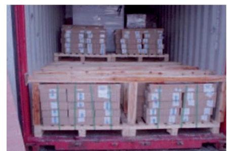
Temporary timber floor
