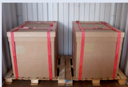
Cargo firmly secured to pallets by textile lashings
