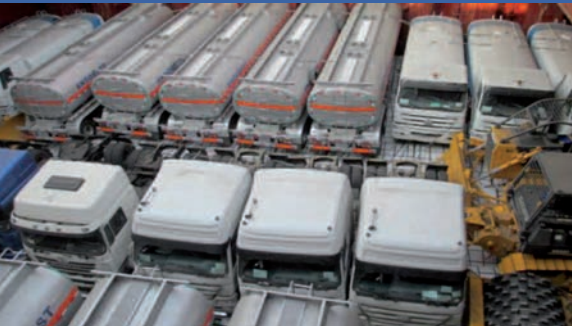
Proximity stowage of vehicles stowed on top of cement cargo
