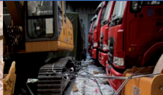
Inadequate separation, securing and lashings
