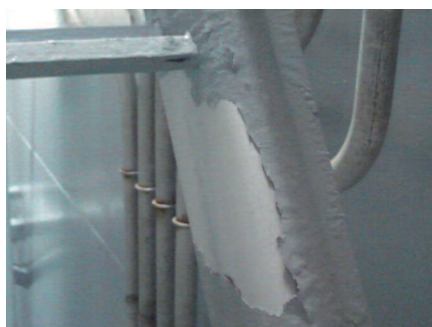
液货舱涂层因过热受损
