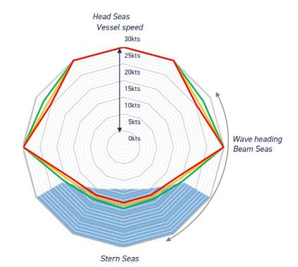
To reduce the risk of large roll motions, IMO guidance recommends changing the vessel heading or adjusting the speed, whilst avoiding abrupt steering. The guidance in the following pages shows, for a range of generic containership vessel sizes and typical loading conditions, the expected safe zone where dangerous situations are less likely to occur.
