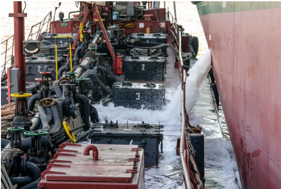
Beware what is alongside before de-ballasting
