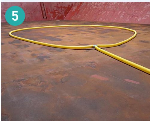
Figure 5: Yellow pipes used for fumigation inside cargo hold
