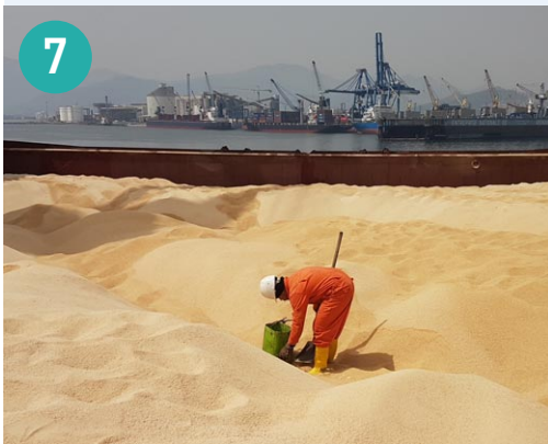
Figure 7: Crew collecting damaged cargo from a cargo hold after gas-freeing
