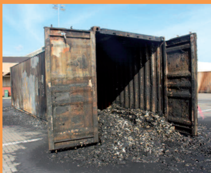
Discharge of a container of charcoal showing how charcoal can re-ignite with burning material falling through the floor of the container.
