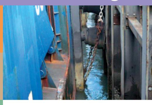
When deciding the ship's berthing position it is important to consider the location of port property (such as fenders) and how they are positioned in relation to any protrusions or recesses on the ship's hull. It is not just the more obvious parts of the hull such as the protruding bow flare or bridge wings that should be considered, but other less obvious areas.
