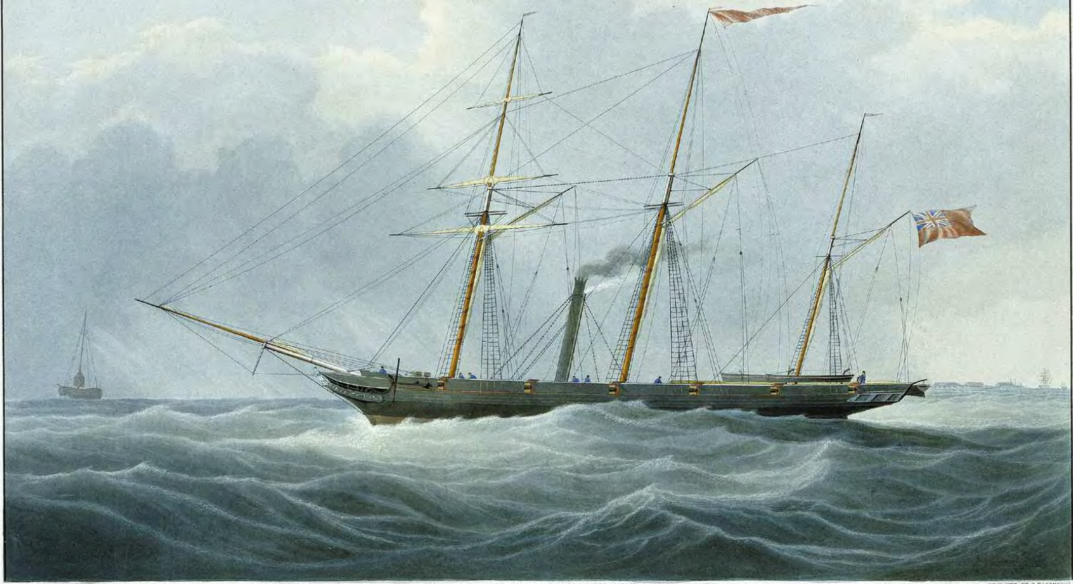
PAINTED BY W. J. HOPKINS. LONDON: PUBLISHED BY MR. HUGGINS, MARINE PAINTER TO HIS LATE MAJESTY WILLIAM IV. 10, LEADENHALL STREET. EXECUTED BY C. ROBINSON. THE ARCHIMEDES, FITTED WITH MESSRS. SMITH'S PATENT SCREW PROPELLER. OFF THE COAST, ON HER TRIP FROM GRAVESEND TO PORTSMOUTH, WHICH WAS PERFORMED IN 21 HOURS, AGAINST A FRESH BREEZE FROM THE WEST—MAY 18 TH 1839. STEAMER. Built by M. H. Wanshurst of Limehouse, for the Ship Propeller Company. JAMES'S GATE S. EXTREME LENGTH 125 FEET DRAUGHT OF WATER FORWARD 9 FEET LENGTH BETWEEN PERPENDICULARS 107 DO. BURTHEN IN TONS 250 TONS. EXTREME BREADTH 22 - 6 IN. UNITED POWER OF ENGINE 250 HORSE. DEPTH OF HOLD 13 DO. DIAMETER OF SMOKE 5 FT 6 IN. DRAUGHT OF WATER AFT 10 DO. LENGTH OF DECK 5 FT
