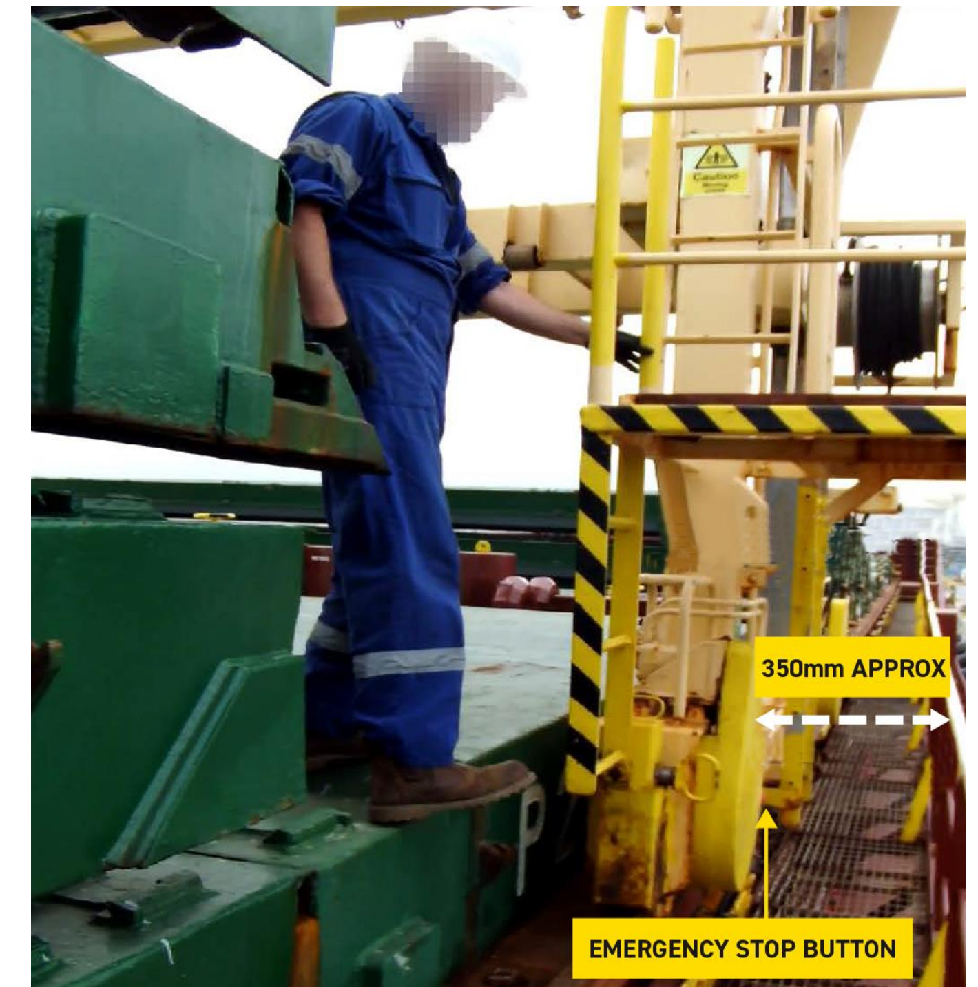
Access to starboard emergency stop button
