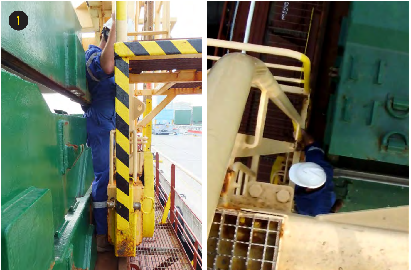
FIGURE 1 RECONSTRUCTION SHOWING A CREW MEMBER IN THE GAP BETWEEN THE LADDER PLATFORM AND STACKED HATCH COVERS. SOURCE: MARINE ACCIDENT INVESTIGATION BRANCH (MAIB), © CROWN COPYRIGHT, 2020
