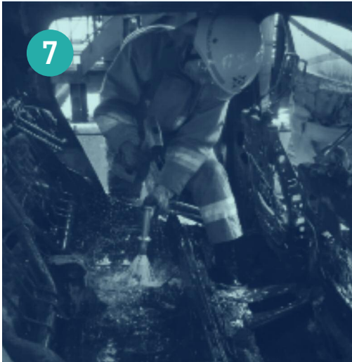
A firefighter spraying water into a battery pack during overhaul of a burnt EV. Reproduced with kind permission of NYK
