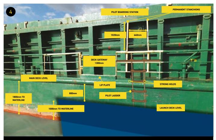
FIGURE 4 REPRODUCED IMAGE OF CARGO VESSEL'S DECK GATE AND PILOT BOARDING ARRANGEMENTS SOURCE MARINE ACCIDENT INVESTIGATION BRANCH – GOV.UK: ANNUAL REPORT 21/2017
