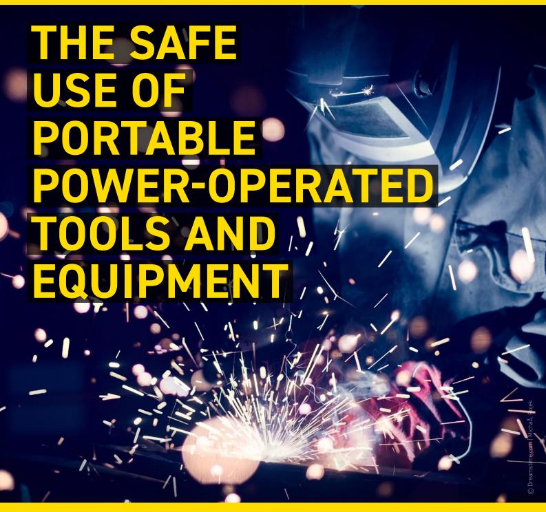
THE MAIN ISSUES IDENTIFIED ARE THE REMOVAL OF SAFETY SLEEVES FROM NEEDLE SCALERS, THE REMOVAL OF SAFETY GUARDS, OR THE INEFFECTIVE MODIFICATION OF SAFETY GUARDS. INDIVIDUALS HAVE ALSO BEEN TAMPERING WITH OR BYPASSING SAFETY CUT-OUT DEVICES ON TOOLS, USING METHODS LIKE WIRING, TAPING OR OTHER MEANS. ELECTRIC TOOLS SIMILARLY SUFFER FROM POOR GENERAL MAINTENANCE, INCLUDING WIRING FAULTS.
