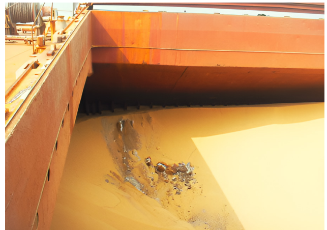
FIGURE 7 Evidence of water ingress at the cargo hold entrance hatch and the hatch coaming
